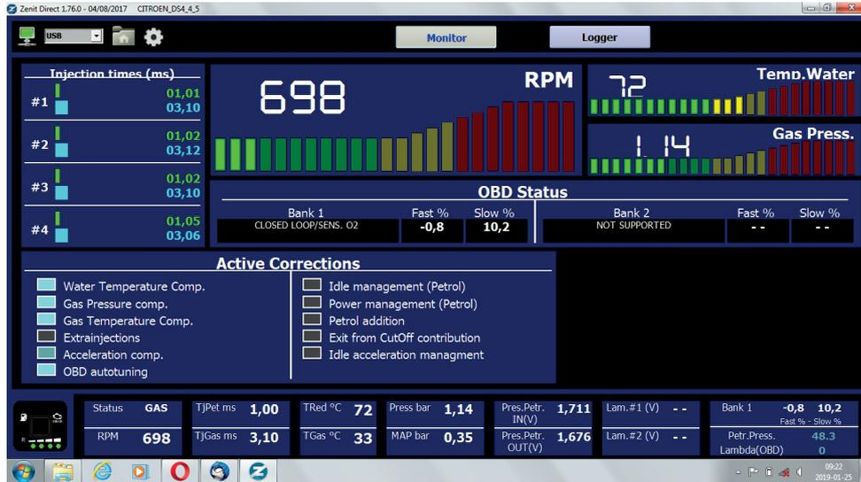
This tab allows to monitor the most important parameters and active functions of the system.
