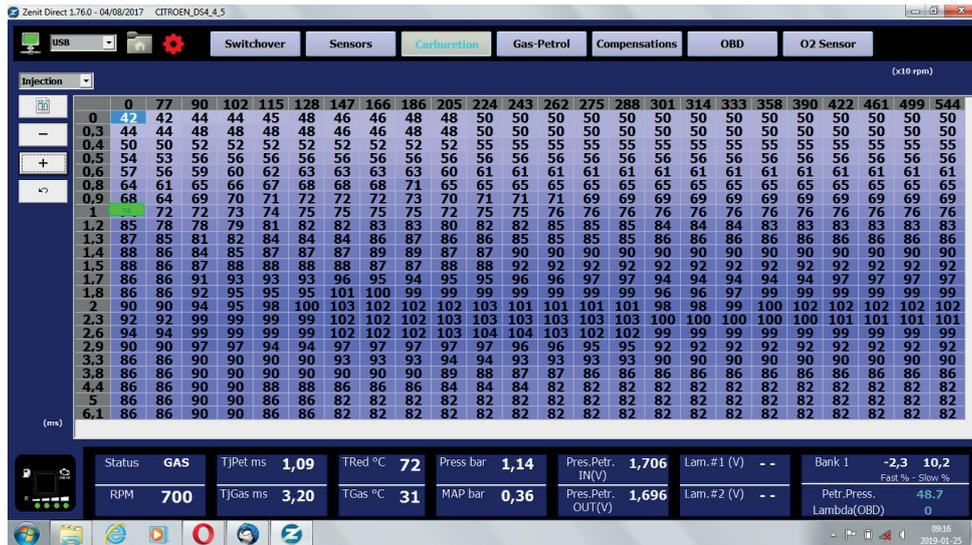
This tab contains a map that allows to adjust the gas dose depending on the opening times of petrol injections and engine speed.
