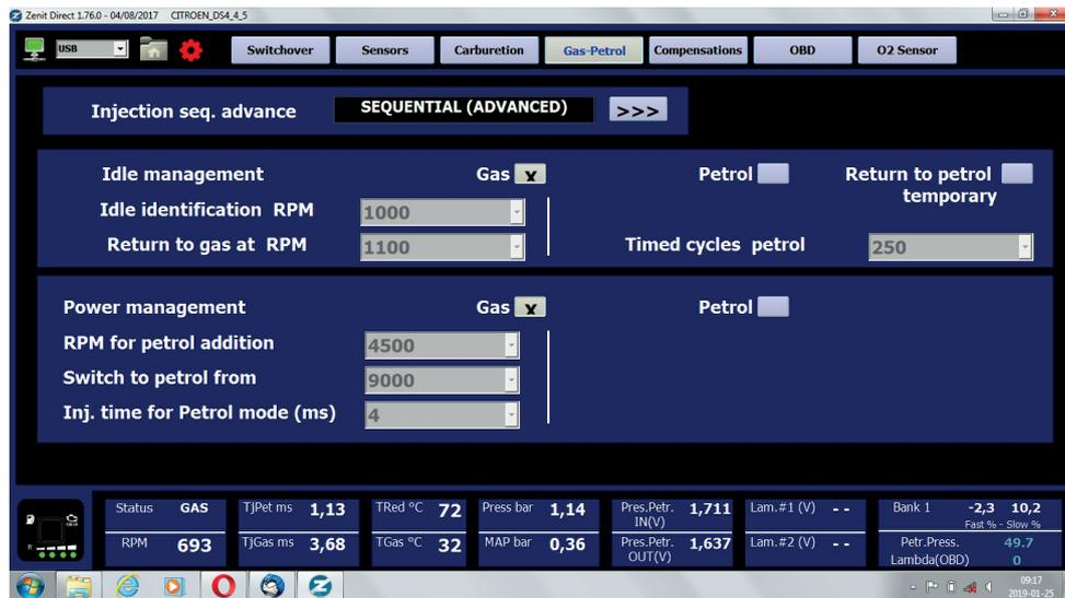
In this option, it is possible to set the switching only to gasoline supply for low and high revolutions (engine speed).
