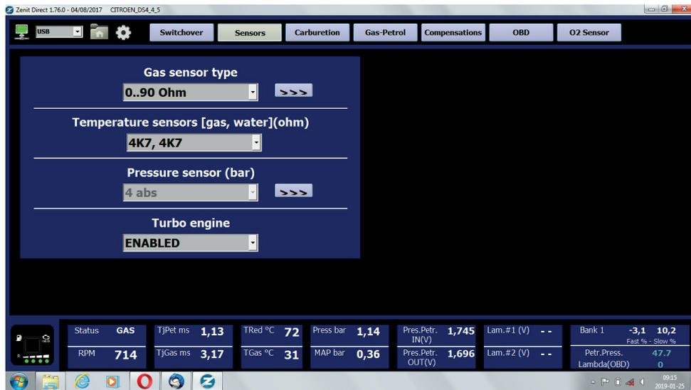
**Type of the gas level sensor** - gives the possibility to choose the sensor type which is installed in the system. The button on the right side activates the calibration window of the gas level sensor. This calibration consists in setting the voltage thresholds above which the individual diodes should light up. For this purpose, move the slider to the left or right to set the required value.
