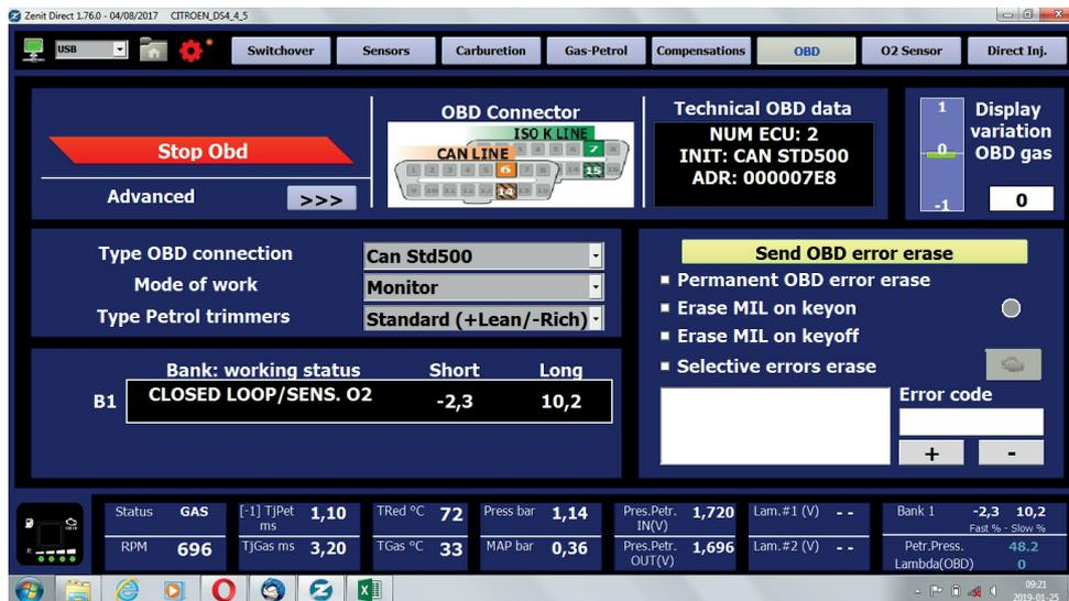
**OBD type** - should be set automatically when activating the connection to the OBD system. It is also possible to manually change the communication protocol in case of problems with correct automatic detection.
