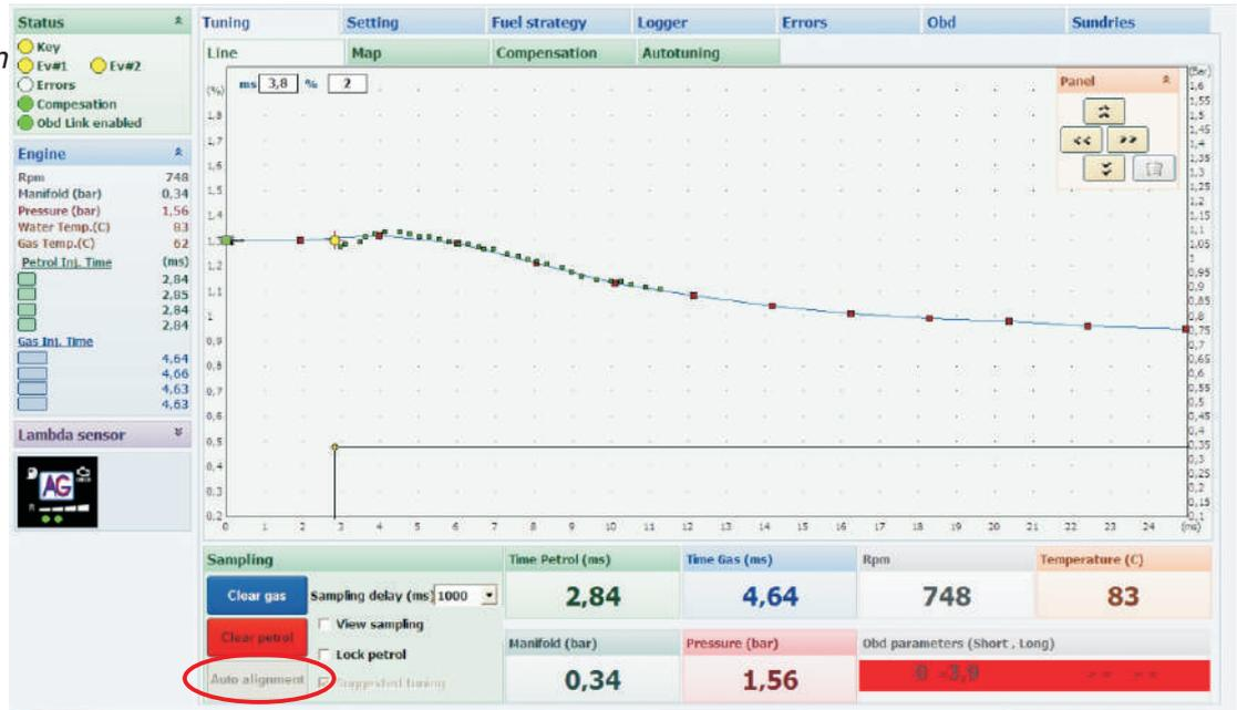
After adjusting the model you have to collect the gas map again. To do this, select the option **View sampling**. Only the petrol map will appear as the gas map is automatically deleted. A new map of the gas is made in the same way as the previous one.
