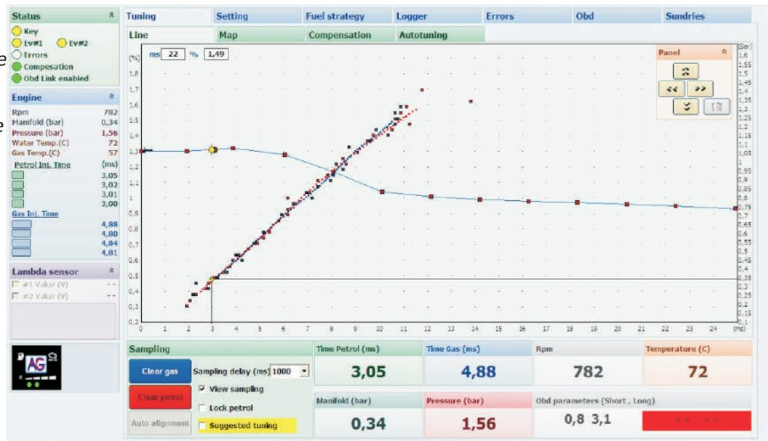
When there are discrepancies, the correction procedure should be performed. We do this by selecting the **Suggested tuning** (this option activates automatically and highlights in yellow when we collect a sufficient number of map points).
