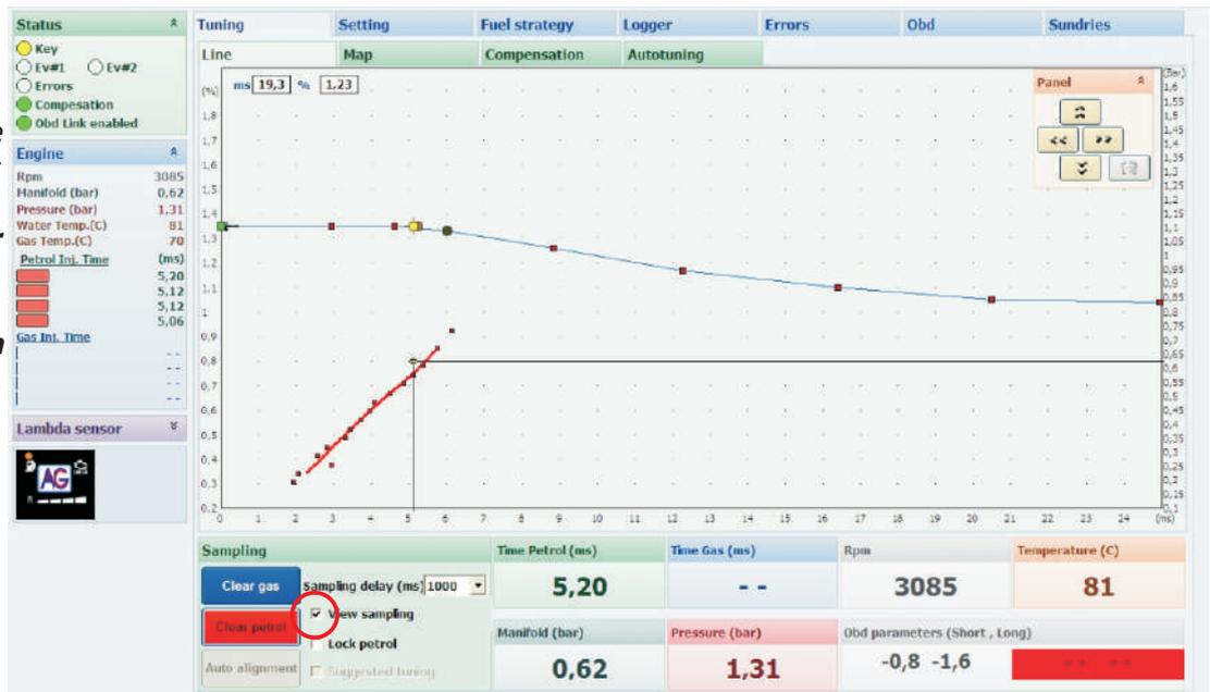
If the points are visible in the whole range of engine loads and the dotted line is visible you can start creating the gas map.
