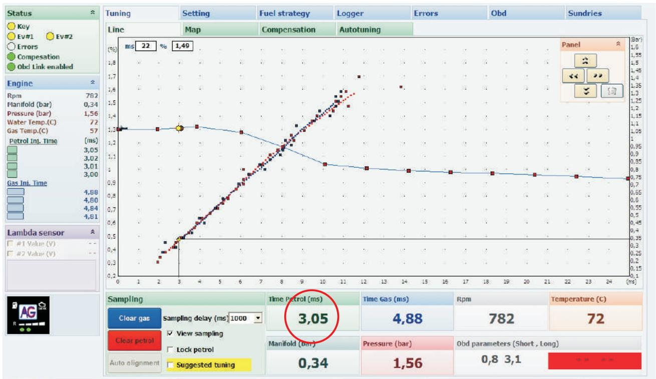
In the example above, the petrol injection time at low rpm is 3.05 ms. After changing to gas supply, the time should be within 3% error which should be from 2.95 to 3.13. If this difference is greater, it must be corrected by setting using the tab **Tuning -> Map**.
