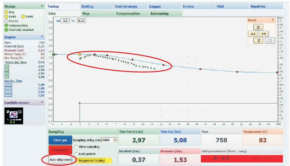
In the automatic option, after pressing the **Auto alignment**, the program will correct the model itself.
