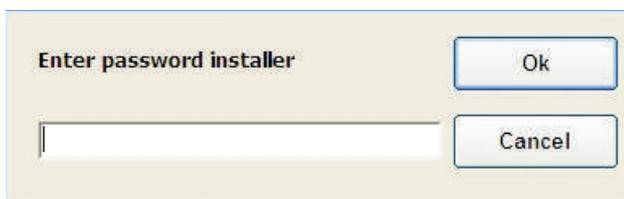
After entering the correct password and pressing **Ok.**, the system will be unlocked and you can make configuration changes. If the password is forgotten or unknown, it is possible to restore the system to factory settings and remove the password. To do this, click the **Cancel** button and the window will appear.
