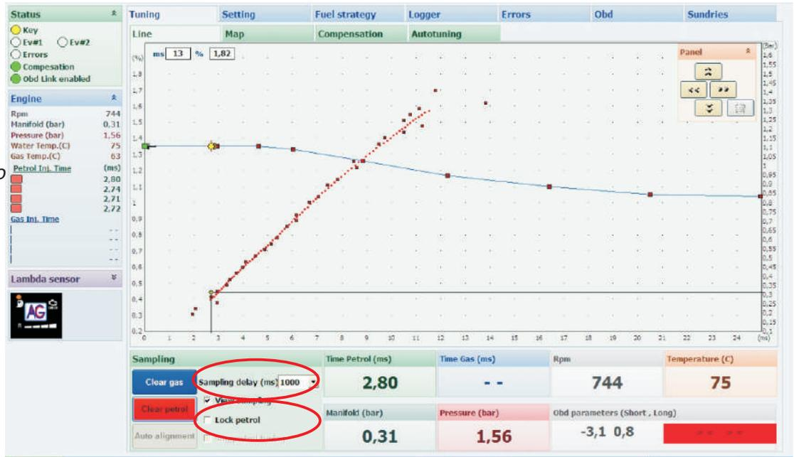
After creating a petrol map, switch system to gas and create a **gas map** in exactly the same way as petrol one.
