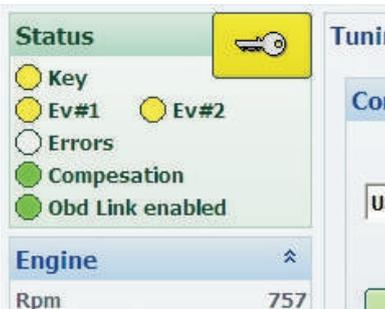
To make changes to the system settings, click on the button with a key symbol and then a window appears to enter a password and temporarily unlock the system (until you disconnect from the ECU)
