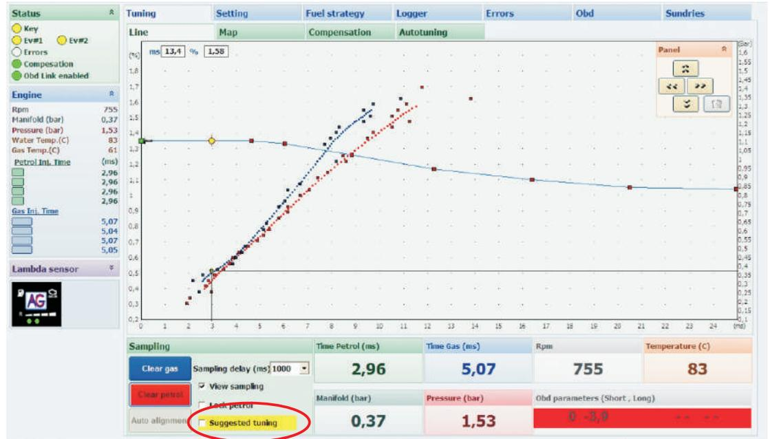
On the chart there will appear green points suggesting what the model should look like for the petrol and gas maps to overlap. At this point, the model must be adjusted. You can do this in two ways: using the automatic **Auto alignment** function or you can do it manually. Deciding for manual adjustment, by "pulling" individual regulatory model points you lead a line as close as possible to the green points, gently, with no sudden curves.
